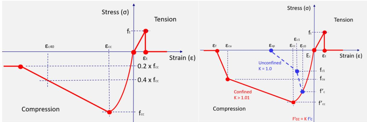
Figure 3. Different Concrete models implemented in this study
