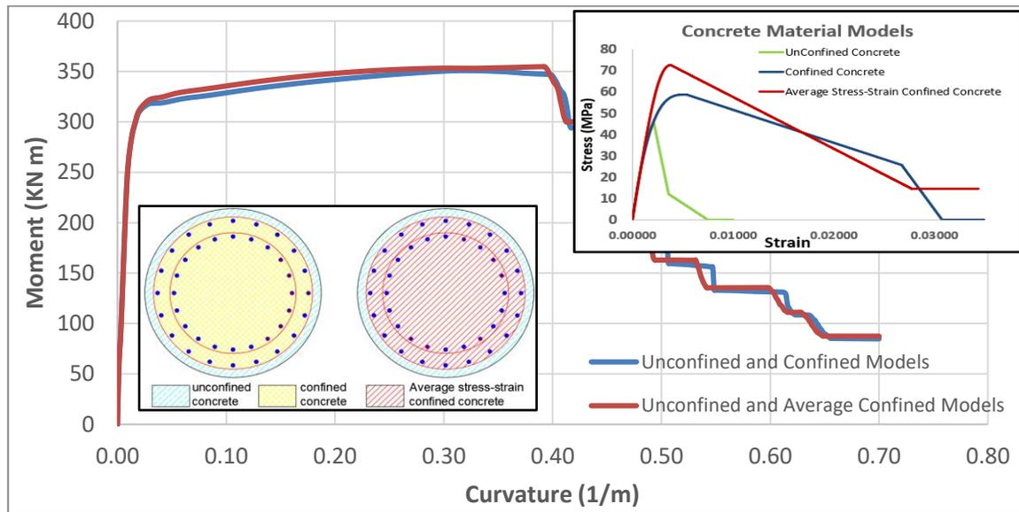
Figure 11. MC (Confined and unconfined concrete vs the average uniform confinement method)
