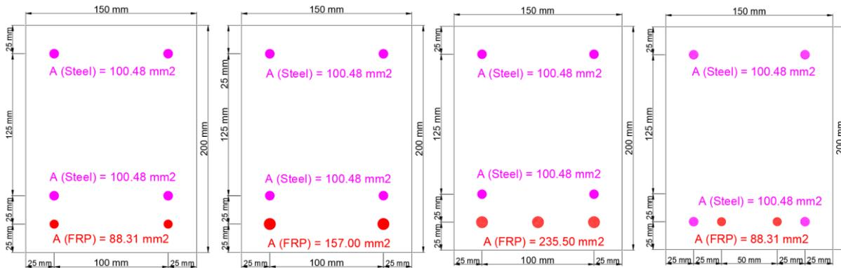
Figure 4. Cross section and reinforcement details
