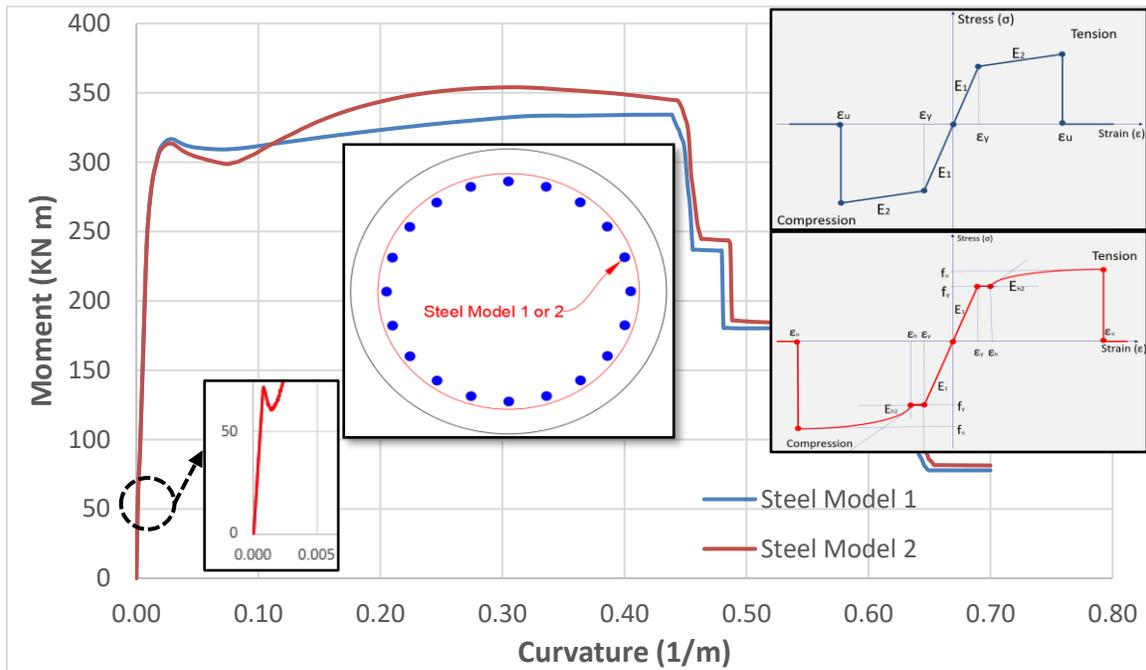
Figure 8. MC (bi-linear steel model vs nonlinear strain hardening steel model)
