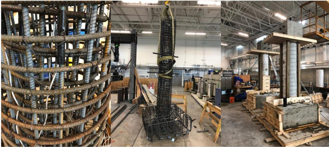
Figure 12. One and two layers of spirals specimens prepared for testing at ALAMS
