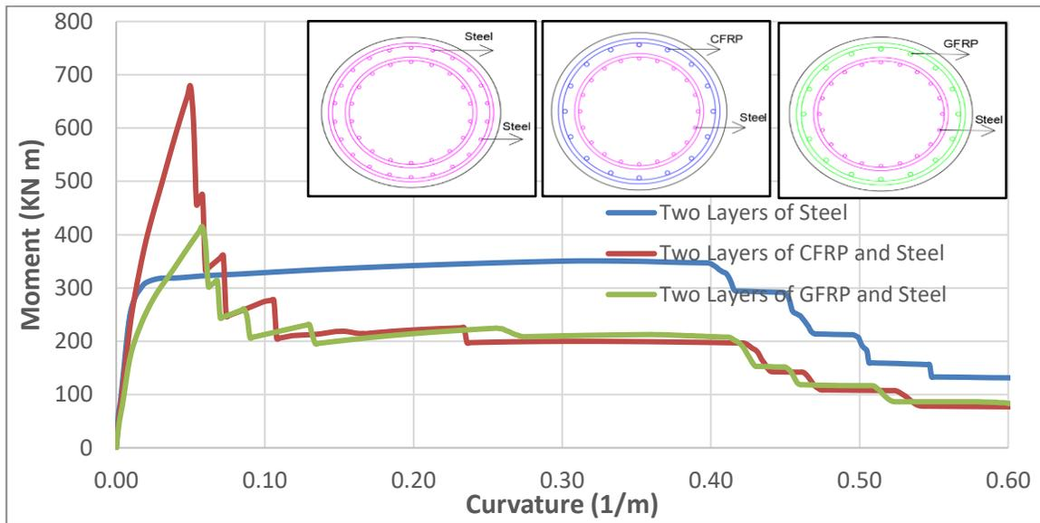
Figure 9. MC (Hybrid-reinforcement utilizing steel, CFRP and GFRP)
