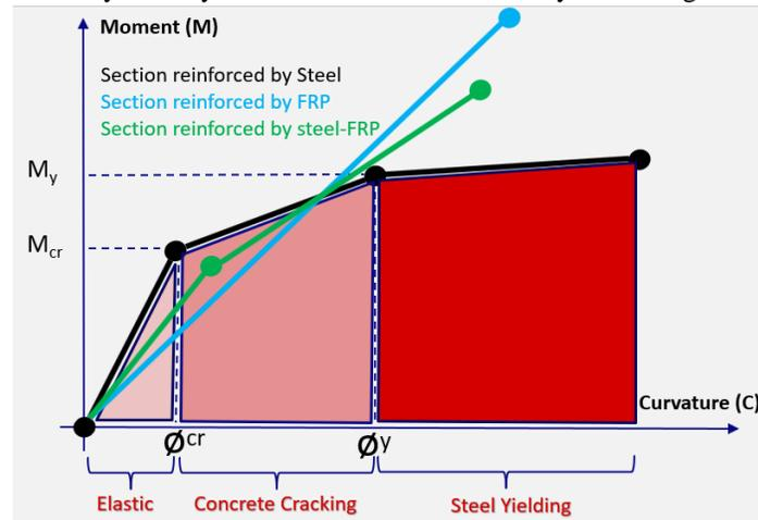
Figure 2. Schematic MC relation of hybrid-reinforced RC sections
