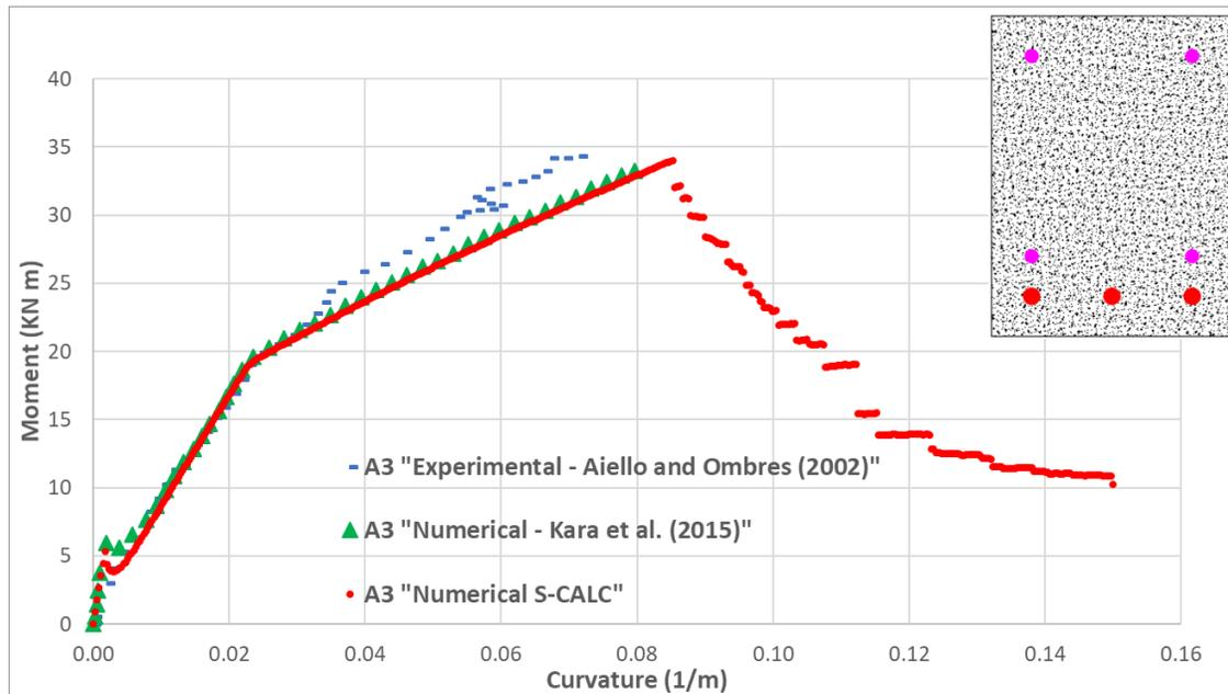
Figure 5. Numerical results validated against both experimental and numerical results from the literature
