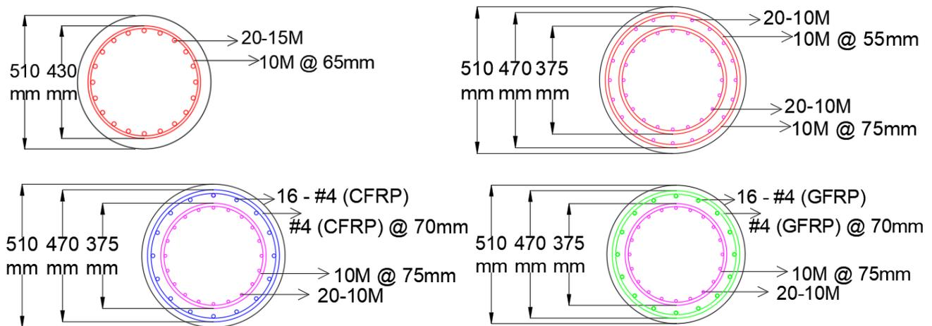
Figure 6. Cross section and reinforcement layout of the scaled models; (a) Steel (Control), (b) two layers of spirals (both Steel), (c) two layers of spirals (CFRP and Steel) and (d) two layers of Confinement (GFRP and Steel)
