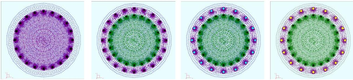
Figure 7. Mesh is tuned to precise element size near rebars while courser mesh is applied in other section parts
